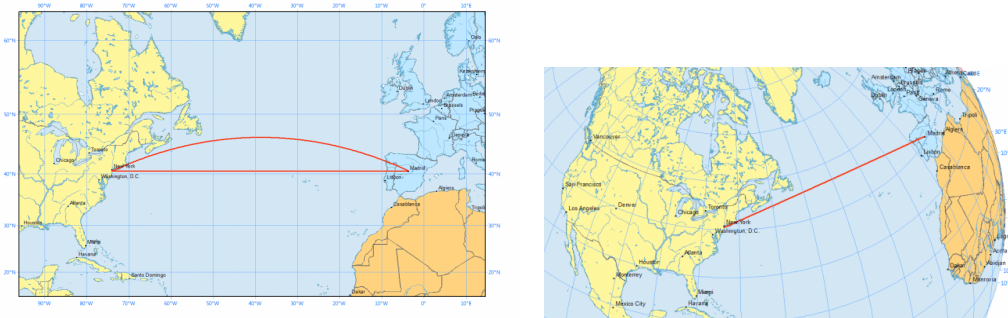
Figure 3: Of the two flight paths seen on the Mercator projection (left), the curved one is actually a shorter distance and is seen again on the right. Source .
